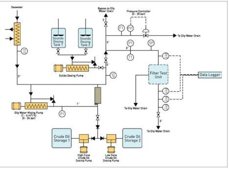
Figure 2 - Test Stand Schematic
