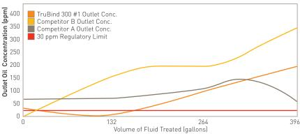
Graph 5 - Competitive comparison mass of oil removed at 5.3 gpm
